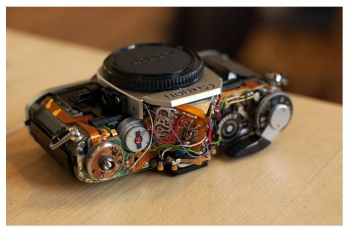
The innards of a Canon AE-1, showing the vast amounts of electronic components – not bad for the 70's!
